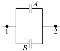
$$\text{On a } Q_{A_1} = -Q_{A_2} = C_A(V_1 - V_2), \quad Q_{B_1} = -Q_{B_2} = C_B(V_1 - V_2)$$
