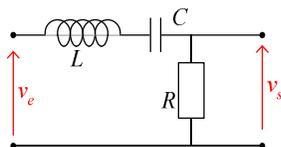
$$\underline{H}(j\omega) = \frac{R}{R + j\omega L + \frac{1}{j\omega C}} = \frac{R}{R + j\left(\omega L - \frac{1}{\omega C}\right)}$$
