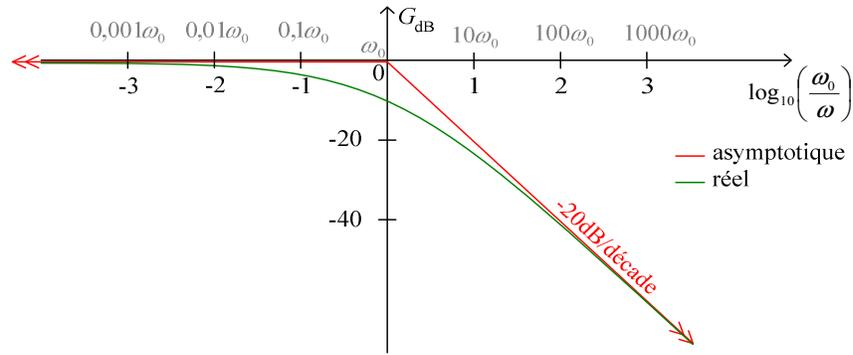
$$G(\omega_0) = \frac{1}{\sqrt{2}} \Rightarrow G_{\text{dB}}(\omega_0) = -3\text{dB}$$
